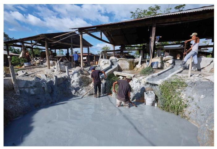
Water is an essential ingredient of artisanal processing, sourced from streams, circulated through the rastras (the preferred processing system used by the locals), and returned to the waterway. Copyright: Calibre Mining Corporation.
