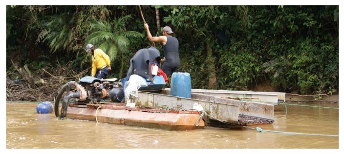
Alluvial miners on the Rio Zarza in south-east Ecuador. A diver guides a suction pump to pull up gravel which then passes over a sluice on the raft. Copyright: Kinross.
